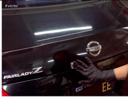
6 Make sure to clean the surface of the installation area and then apply the adhesive promoter along the surface.
