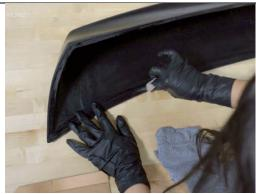
1 Sand down the tape line area. This will remove any mold release left over from the mold.
