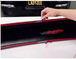
5 Slightly peel off the ends of the 3m tape. This will help you center the spoiler before fully attaching it.
