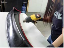
4 Use a heat gun to create flexibility. This allows the ducktail to easily mold onto the trunk of the vehicle.
