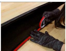
3 Now, start applying the 3m double sided tape along the tape line of the Vicrez ducktail.
