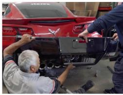
1 Remove the C7 rear bumper fascia. This will facilitate the installation process.
