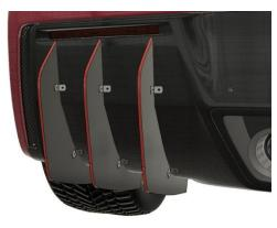
4 Align the fins to the surface of the rear facia and mark the holes with an easy to remove marker.
