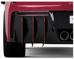
Peel off the 3M tape backing and apply firm pressure to tape locations to ensure proper adhesion.
