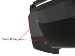
**5** Drill the holes for the rear add-on fins and the rear facia where you have previously marked.
