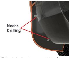
**5** Drill the holes for the rear add-on fins and the rear facia where you have previously marked.
