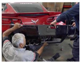
Remove the C7 rear bumper fascia. This will facilitate the installation process.
